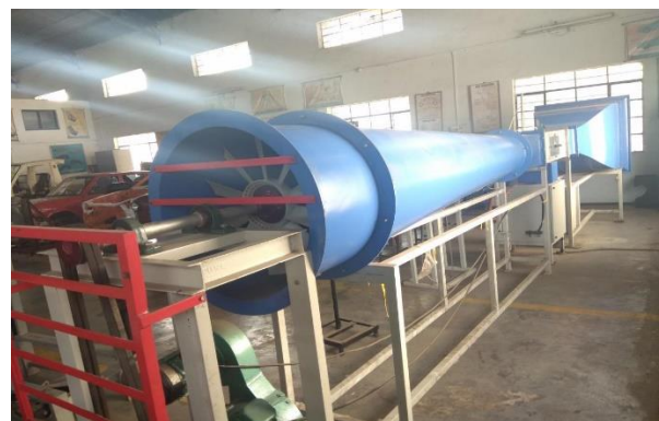
Fig 1 Open circuit wind tunnel used for experimental investigation
