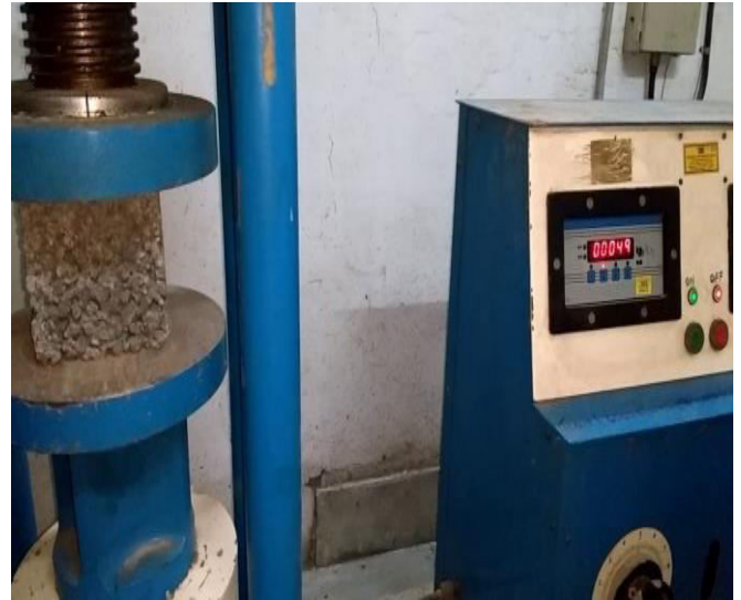
Figure 6. Compressive strength tests
