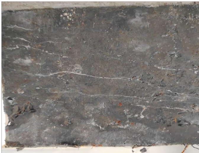
Figure 8 : Self Healing of Cracks
