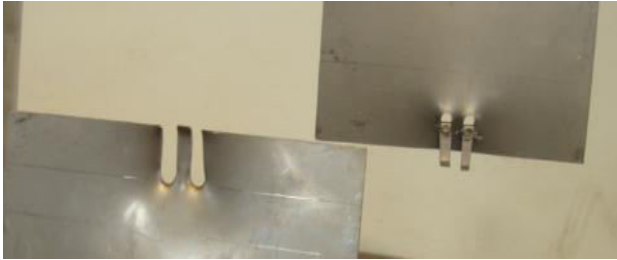
Fig.6 .Pull out failure mode
