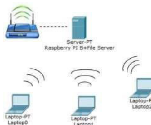
Figure 1 System Architecture of client/server files sharing
