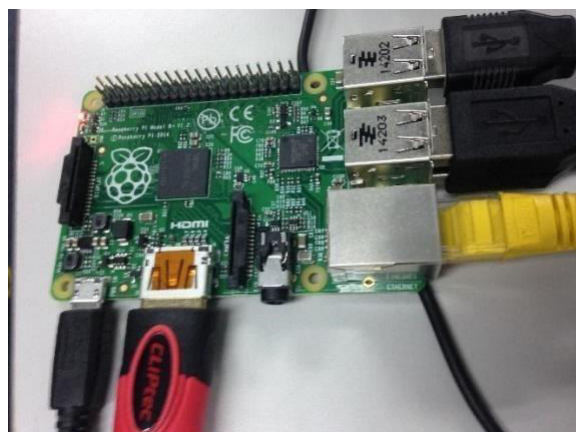
Figure 6: Raspberry Pi model B+ connected to HDMI, Mouse, Keyboard, LAN and XBee (USB)
