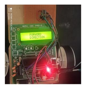
**Expected Result :** The Position of iris and pupil will be detected and and produced using Viola Jone Algorithm.After that they are processed using MATLAB. Then decision will be taken by Microcontroller for the given input image. as per the pupil movement motor will be moved either in left,right,forward and backward direction.
