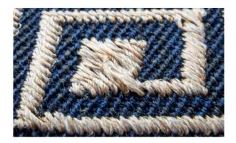
Fig. 4: Embroidered conductive pattern on the textile substrate
