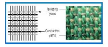
Fig.2 Conductive yarns in the fabric structures
