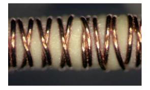
Fig 1. Elastic electroconductive yarn
