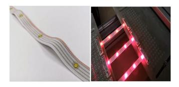
Fig. 5 Conductive stretchable textile ribbons with integrated LED and these ribbons after 4500 stretching cycles[16]
