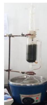
Fig.4 Extraction process using Soxhlet Apparatus
