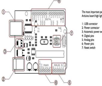
Arduino board high ligh I: USB connector 2: Power connector
