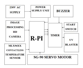
Fig.1: Block diagram of overall project
