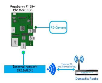
In this Project Raspberry Pi acts as a complete Surveillance and Alarming System. Our goal is to make a self-aware system that recognizes faces easily without a rigorous training system and will be able to stream the results over the internet to alarm the user of activity using Twilio SMS services.
