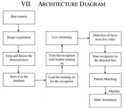
Fig 1. Architecture Diagram
