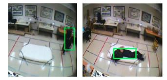
Figure 3.7: Bounding box enclosing target
