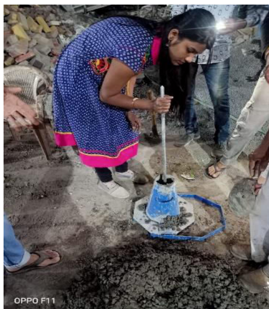
Fig. 4- Performing slump cone test
