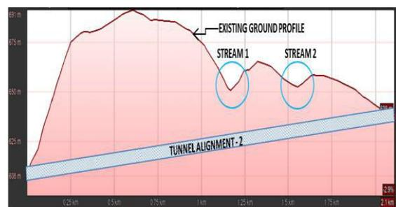
Figure– Longitudinal Profile along tunnel alignment –2
