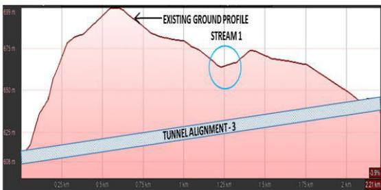
Figure– Longitudinal Profile along tunnel alignment – 3
