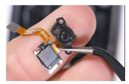
Optical reflexive fingerprint scanning device
