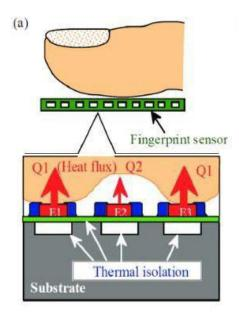
E1, E2 and E3: arrayed heater elements
