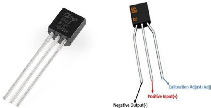
A temperature sensor is an electronic device that measures the temperature of its environment and converts the input data into electronic data to record, monitor, or signal temperature changes.
