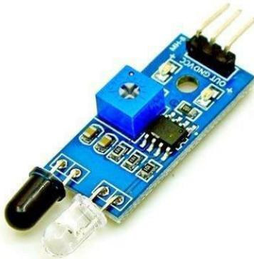
The emitter is an IR LED and the detector is an IR photodiode. The IR photodiode is sensitive to the IR light emitted by an IR LED. The photo-diode's resistance and output voltage change in proportion to the IR light received.
