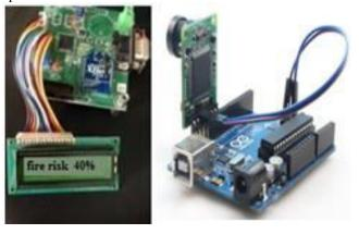
Figure 1. Sensor node and Video node
