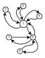
Figure- Functional Graph of flexible manufacturing system 1 – conveyor, 2 – storage, 3 – pallet handling and quality station, 4 – robot vision and assembly station, 5 – robot feeder of machine tools, 6 – CNC lathe, 7 – CNC milling machine
