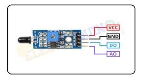
Fig.5 IR Flame Sensor
