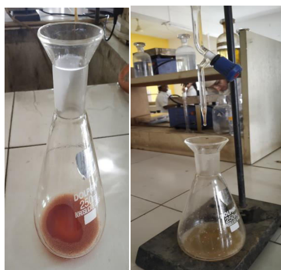
Figure:-Saponification value test with substance
