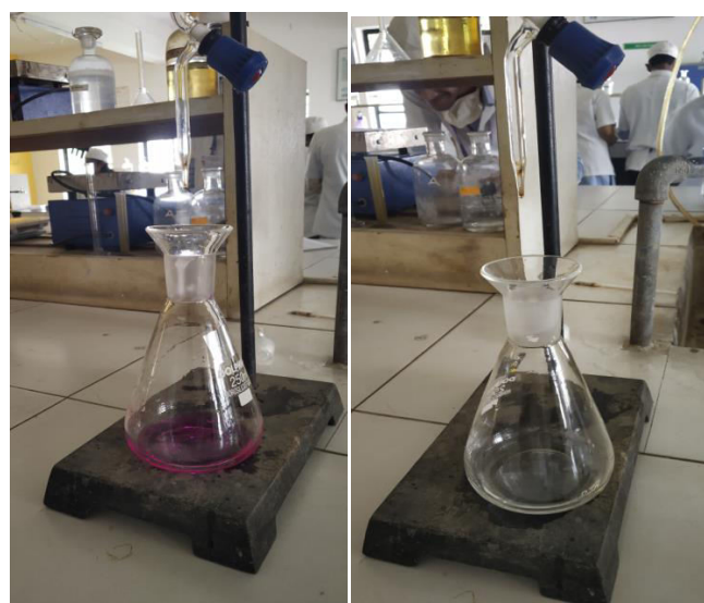
Figure:- Saponification value test with blank
