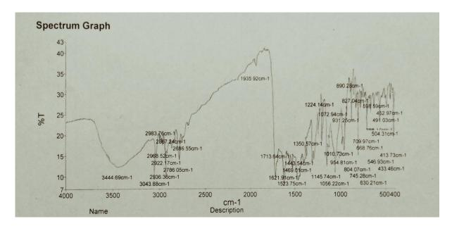
Figure no. 4 : FTIR spectra of pure drug Ofloxacin
