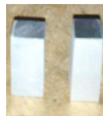
Fig.2. MMC specimen for wear test
