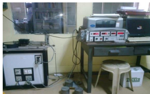
Fig.1. Pin on disc apparatus
