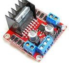
Fig 2.4 Motor driver module (L298N)
