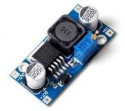
This is a buck-boost converter use for the equalization of the power coming from the solar panels. And it also safeguards the battery from the larger voltage and current.
