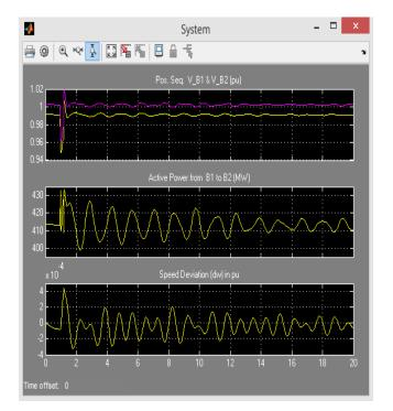
Figure (6) (a) System Response for Single Phase fault condition with PID Controller
