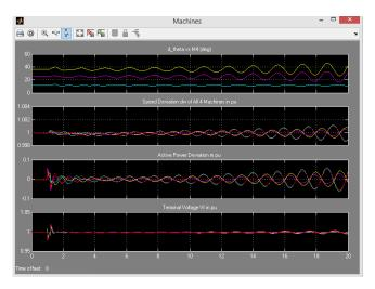
Figure (5) (b) System Response for Single Phase fault condition without PSS
