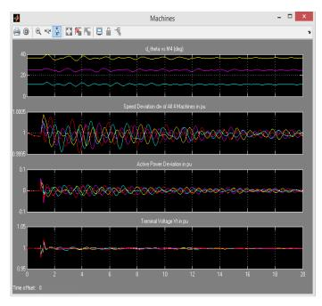
Figure (6) (b) System Response for Single Phase fault condition with PID Controller
