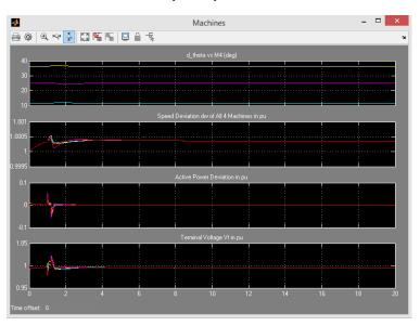
Figure (7) (b) System Response for Single Phase fault condition with Grey Fuzzy PID Controller
