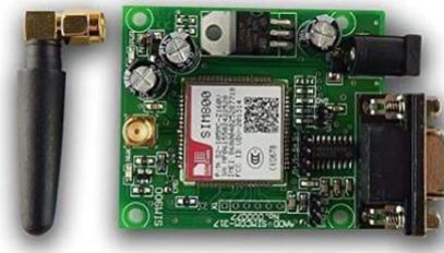
**Fig. 3 GSM(SIM800)**
