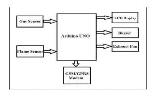
Fig.1 Block Diagram of Gas Detector
