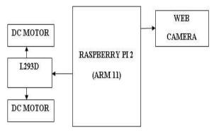
Fig 1. Block diagram of Robot section
