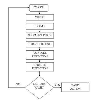
Fig 5. Flow chart of OpenCV Algorithm
