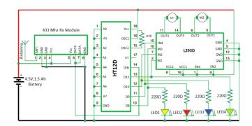
The receiver part consists of 433MHz RF receiver module (RX1), HT12D decoder (IC5) and L293D motor driver (IC6) to run the motors. Here, receiver module RX1 receives the transmitted signal, which is decoded by decoder IC to get the same digital outputs. Four outputs of IC6 drive two motors. The robot moves as per tilt direction of the accelerometer in the transmitter.
