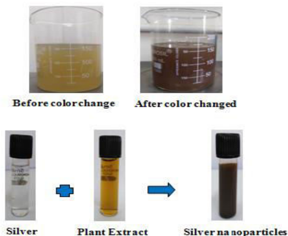
Fig 2 Color change of plant extract after the addition of AgNO 3
