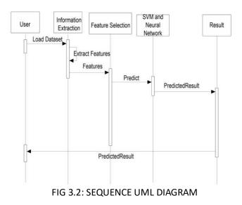
A sequence diagram in Unified Modeling Language (UML) is a kind of interaction diagram that shows how processes operate with one another and in what order. It is a construct of a Message Sequence Chart
