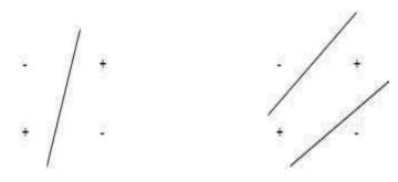
The MultiLayer Perceptron (MLPs) breaks this restriction and classifies datasets which are not linearly separable. They do this by using a more robust and complex architecture to learn regression and classification models for difficult datasets.
