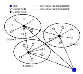
Fig. 1. Architecture of Clustering in WSN
