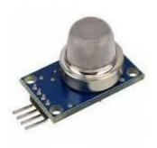
The MQ-6 module is used in gas leakage detecting equipment in family and industry, This module has high sensitivity to LPG, iso-butane, propane and LNG. It can also be used to detect the presence of alcohol, cooking fumes, and cigarette smoke. The module gives out the
