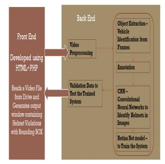
Figure 1: Architecture of Hel Must System
