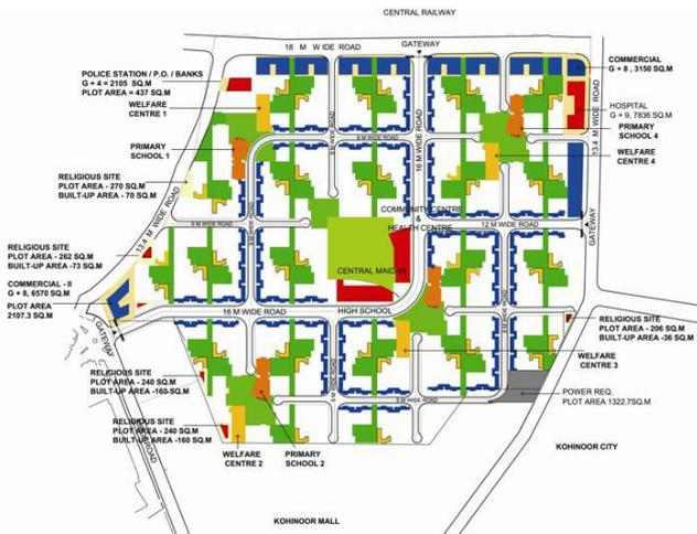
Figure 8 How social infrastructure is planned to easily accessible from building towers (DAS, P K)
