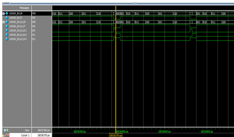
Figure 6 Simulation output for the BPD for different multiplier inputs (Radix-4 Booth algorithm)
