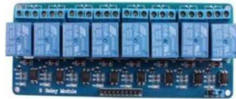
Figure 5: - Relay Board
