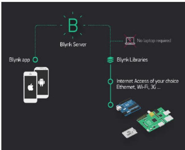
Fig -7: Functioning of the Blynk Application
