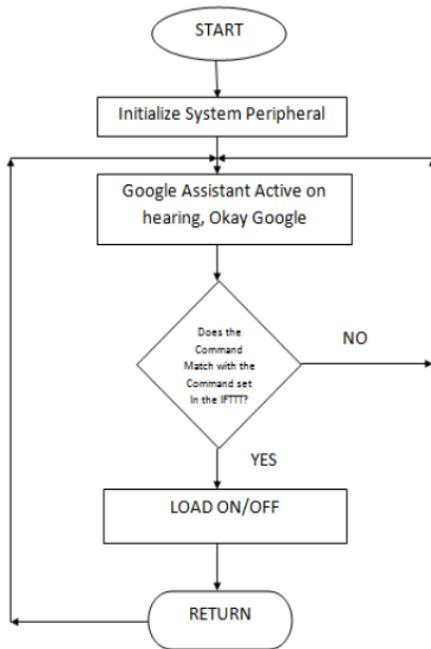
Fig. 3. System Flow Diagram
