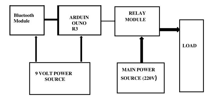
Figure 1: Block Diagram of Home Automation System Using Arduino and Bluetooth Module
