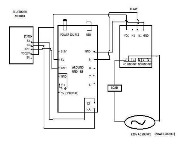
Figure 2: Circuit Diagram of Home Automation System Using Arduino and Bluetooth Module
