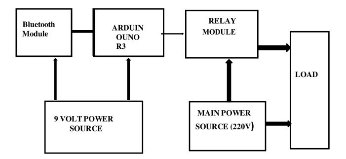
Figure 1: Block Diagram of Home Automation System Using Arduino and Bluetooth Module
