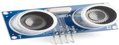
Fig -4: Ultrasonic Sensor
