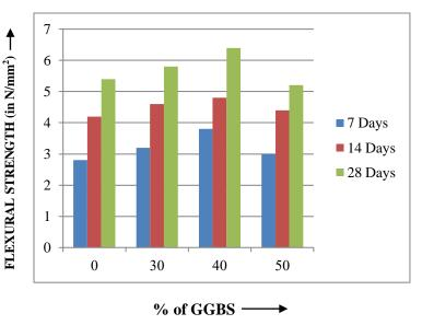
Figure 8: Flexural Strength of concrete v/s % of GGBS
