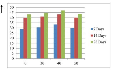
Figure 7: Compressive Strength of concrete v/s % of GGBS
