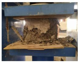
Figure 3: Cube Specimen under Testing
