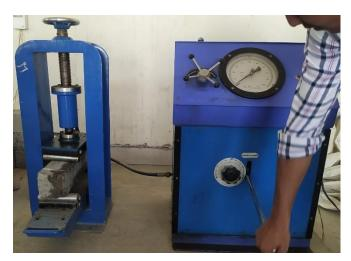
Figure 4: Flexural Testing Machine (Beam specimen under Testing)
