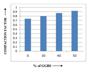
Figure 5: Compaction Factor of concrete v/s % of GGBS
