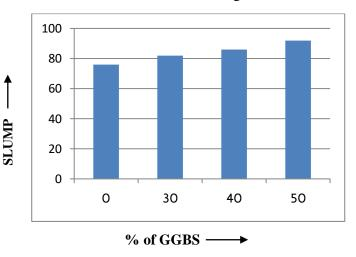
Figure 6: Slump of concrete v/s % of GGBS
