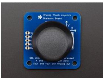
Fig -3: Joystick Module
