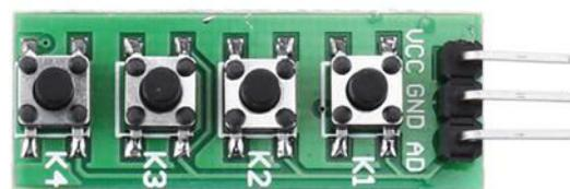
Fig -4: Push Button Switch Module
