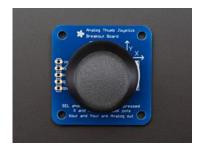
Fig -3: Joystick Module
