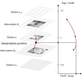
Fig -6: Scale space pyramid for BRISK key-point [9]
