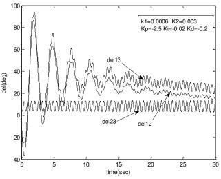
Fig .7 Plot of relative angles with control signal  $K_{p*}error_1+K_i*error_2+K_d*error_3$ .
