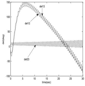
Fig.6.b Plot of relative angles with control signal  $K_p$ \*error<sub>1</sub>+ $K_d$ \*error<sub>3</sub>.
