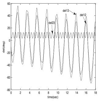
Fig.6.a Plot of relative angles with control signal  $K_p$ \*error<sub>1</sub>+ $K_i$ \*error<sub>2</sub>.
