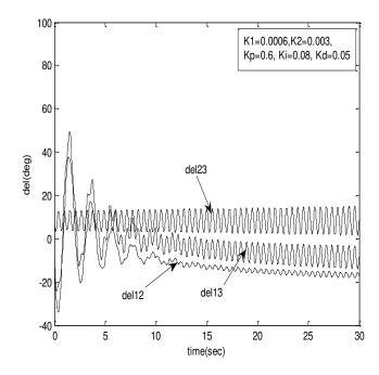
Fig. 8 Plot of relative angles of generators with fuzzy controller
