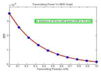
Figure 4(a): For 10 km distance with 09 to 10 mw transmitting power.
