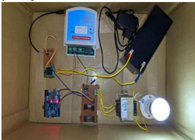
Fig 9 Hardware model: Hybrid inverter and battery charging system
