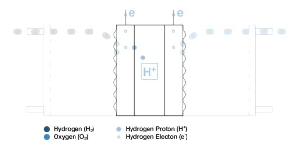
Meanwhile the electrons simultaneously travel through the anode and to an external circuit where they generate electricity and return back to the cathode.
