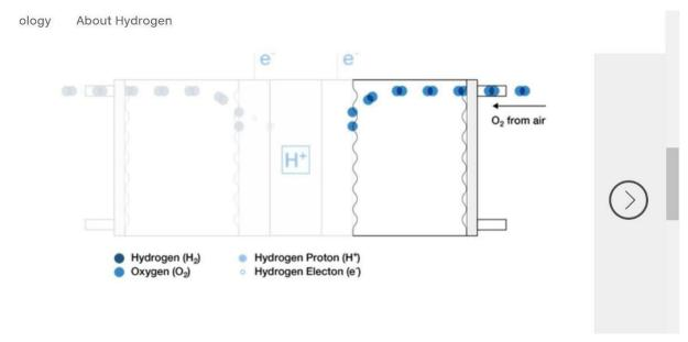
On the other hand at the cathode the oxygen is pulled in and forced through the catalyst, which splits it into two oxygen atoms. These atoms have a strong nega-tive charge thus they attract the positively charged hydrogen ions
