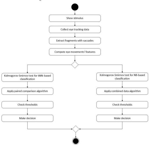
Fig. 8. Scheme of the identification algorithm.
